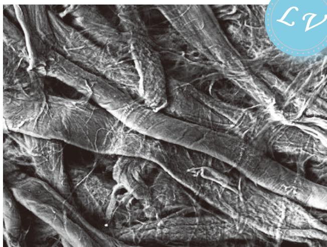
Sample: Paper 50 \mu m Accelerating voltage 15 kV, magnification \times 550
