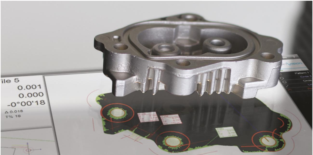
Smart\_Profile\_Matching is an **automatic Profile Check advanced feature**, which can control any item compared to a DXF master. This feature replaces the use of a traditional profile projector that requires the overlay of a glossy sheet on the component's projection.
