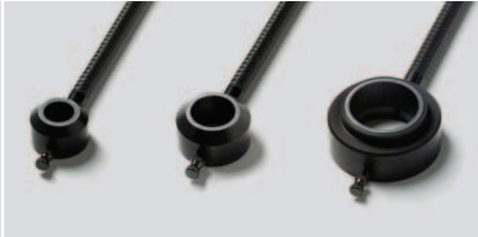
**Standard ringlights** (66 mm with focusing attachment) can be attached directly onto the stereo microscope lens, providing homogenous, shadow-free illumination. They are available as **4-point ringlights** and **continuous ringlights** with a range of long, flexible leads. Adapter 66/58 mm and other adapters for different lens diameters are also available.
