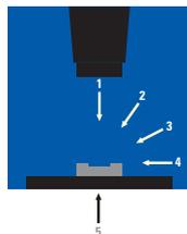
**THE TYPE AND DIRECTION** of the illumination are critical for the outcome. Three approaches are used for the desired optimum image contrast: Incident light (offers highest light intensity with maximum flexibility and greatest selection of lamps), dark field ringlight and transmitted light.
